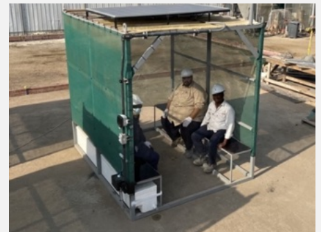
Solar powered sheds used on site, with integrated mist system and cooler.
