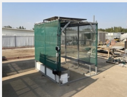
Solar powered sheds used on site, with integrated mist system and cooler.
